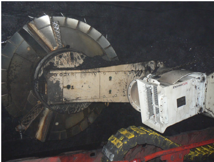
Fig.3. Dust scrubber installed on a longwall shearer
