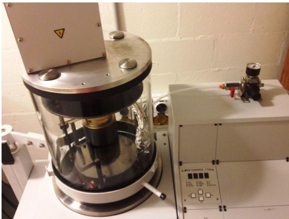
Figure 2. 11: Photograph of EDWARDS FTM6 sputter coater.
