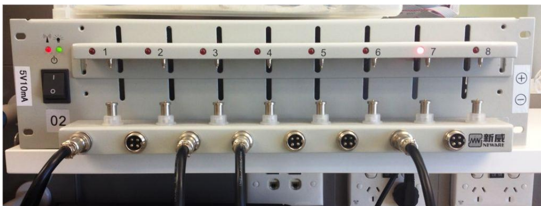
Figure 2. 14: Photograph of Neware cell tester.
