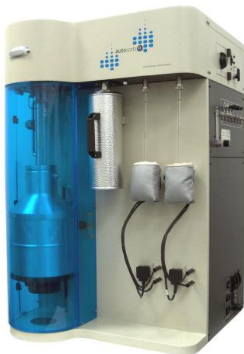
Figure 4. 3: Photograph of BET system used for surface area determination of GO and mw rGO.
