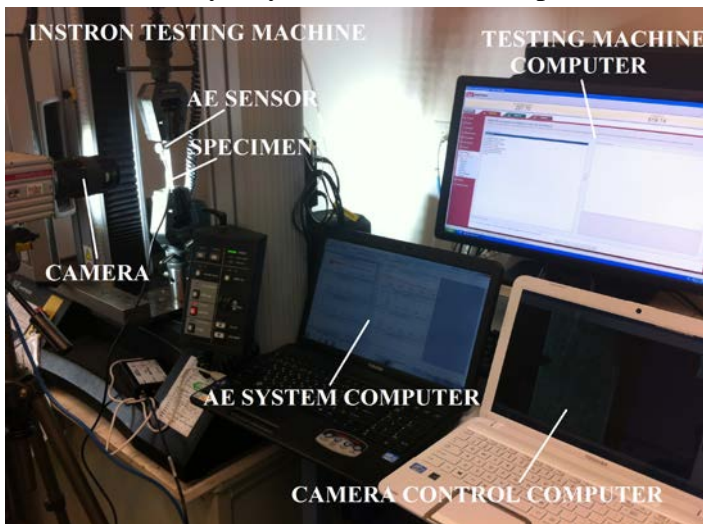
Fig. 2 The experimental setup of the tensile testing
