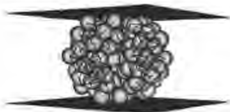
Figure 17. Final fracture of a typical 0.5 mm diameter agglomerate showing intact contact bonds (after McDowell and Harireche 2002).
