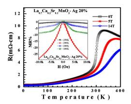
FIG. 4. (Color online) Resistivity plots of  $La_{0.7}Ca_{0.2}Sr_{0.1}MnO_3$ :  $Ag_{0.2}$  under applied field of 0, 7, and 14 T. Inset shows MR percent of  $La_{0.7}Ca_{0.2}Sr_{0.1}MnO_3$ :  $Ag_{0.2}$  at fixed temperatures of 100, 200, 300, and 350 K.
