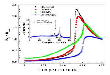
FIG. 2. (Color online) Normalized R(t) plots of  $La_{2/3}Ca_{1/3}MnO_3:Ag_{0.4}$ ,  $La_{0.7}Ca_{0.25}Sr_{0.05}MnO_3$ ,  $La_{0.7}Ca_{0.2}Sr_{0.1}MnO_3$ , and  $La_{0.7}Ca_{0.2}Sr_{0.1}MnO_3:Ag_{0.2}$ . Inset shows the TCR percent as a function of temperature for  $La_{2/3}Ca_{1/3}MnO_3:Ag_{0.4}$  and  $La_{0.7}Ca_{0.2}Sr_{0.1}MnO_3:Ag_{0.2}$ .
