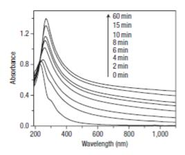
**Figure 4** UV-vis absorption spectra showing the change of GO dispersions as a function of reaction time. The absorption peak of the GO dispersion at 231 nm gradually redshifts to 270 nm and the absorption in the whole spectral region (>231 nm) increases with reaction time, suggesting that the electronic conjugation within the graphene sheets is restored upon hydrazine reduction.
