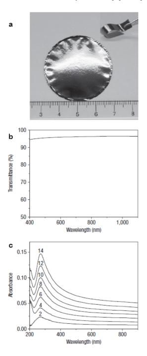
Figure 5 Examples demonstrating that films made of CCG sheets can be easily fabricated from CCG dispersions using various solution-phase processing techniques. a, A 10-µm-thick CCG film or paper prepared by vacuum filtration of a CCG dispersion through an alumina membrane. The film exhibits a shiny metallic lustre. A CCG strip (top-right inset) cut from the film is bent to demonstrate
