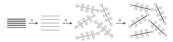
**Figure 1** Scheme showing the chemical route to the synthesis of aqueous graphene dispersions. 1, Oxidation of graphite (black blocks) to graphite oxide (lighter coloured blocks) with greater interlayer distance. 2, Exfoliation of graphite oxide in water by sonication to obtain GO colloids that are stabilized by electrostatic repulsion. 3, Controlled conversion of GO colloids to conducting graphene colloids through deoxygenation by hydrazine reduction.
