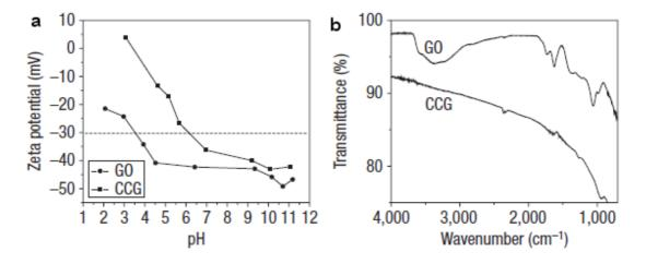
**Figure 2** Surface properties of GO and CCG. **a,** Zeta potential of GO and CCG as a function of pH, in aqueous dispersions at a concentration of ~0.05 mg ml<sup>-1</sup>. **b,** FT-IR spectra of GO and CCG. The absorption band at around 1,700 cm<sup>-1</sup> is attributed to carboxyl groups. The absorption of CCG sheets at this range is observable but not as prominent as that observed for GO, likely due to the overlapping of the strong absorption of graphene sheets in this region.
