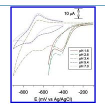
Figure 8. Cyclic voltammetry of 1 mM  $[Cu(Me_8tricosaneN_6)]^{2+}$  (0.1 M aqueous NaNO<sub>3</sub>, 100 mV s<sup>-1</sup> sweep rate) at different pH values.
