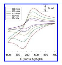
Figure 7. Cyclic voltammetry of  $[Cu(Me_8tricosaneN_6)]^{2+}$  (0.1 M aqueous NaNO<sub>3</sub>, pH 7) at different sweep rates (20 to 500 mV s<sup>-1</sup>).
