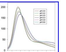
Figure 5. Spectrophotometric (vis–NIR) pH titration of  $[Cu(Me_{8}-ticosaneN_{6})]^{2+}$  in water (0.1 M KNO<sub>3</sub>). The pH values are shown in the legend.
