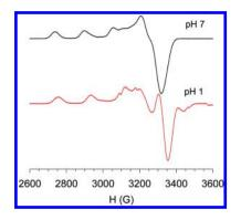
**Figure 6.** X-band EPR spectra of (A)  $[Cu(Me_8tricosane)]^{2+}$  (pH 7) and (B)  $[Cu(HMe_8tricosane)]^{3+}$  (pH 1). Both solutions contained 2 mM complex in DMF/water (1:2), and spectra were acquired at 140 K. The spectral frequency was 9.337 GHz.
