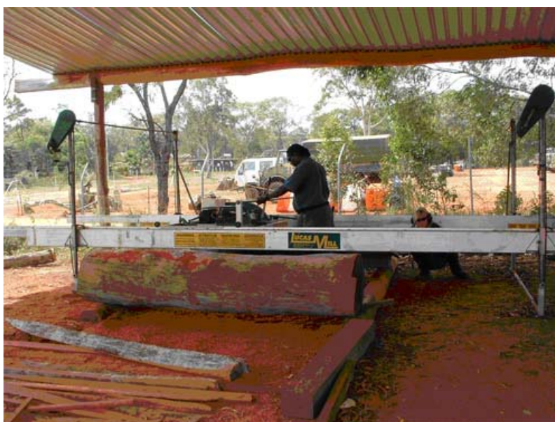
Figure 4: Operating the mobile sawmill at Nanum Tawap, Cape York, 2005. Photo: Queensland Govt.
