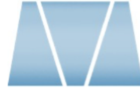
Figure 6: Diagram of the Amici prism used for spectral dispersion.
