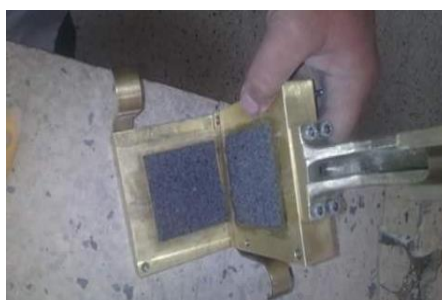
Fig. 11 –Test sample of the mixture M 90-02-08 in shear box before direct shearing
