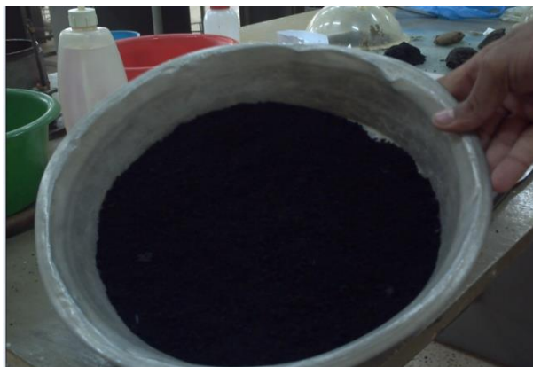
Fig. 4 –Waste tyre rubber powder used in the experimental study
