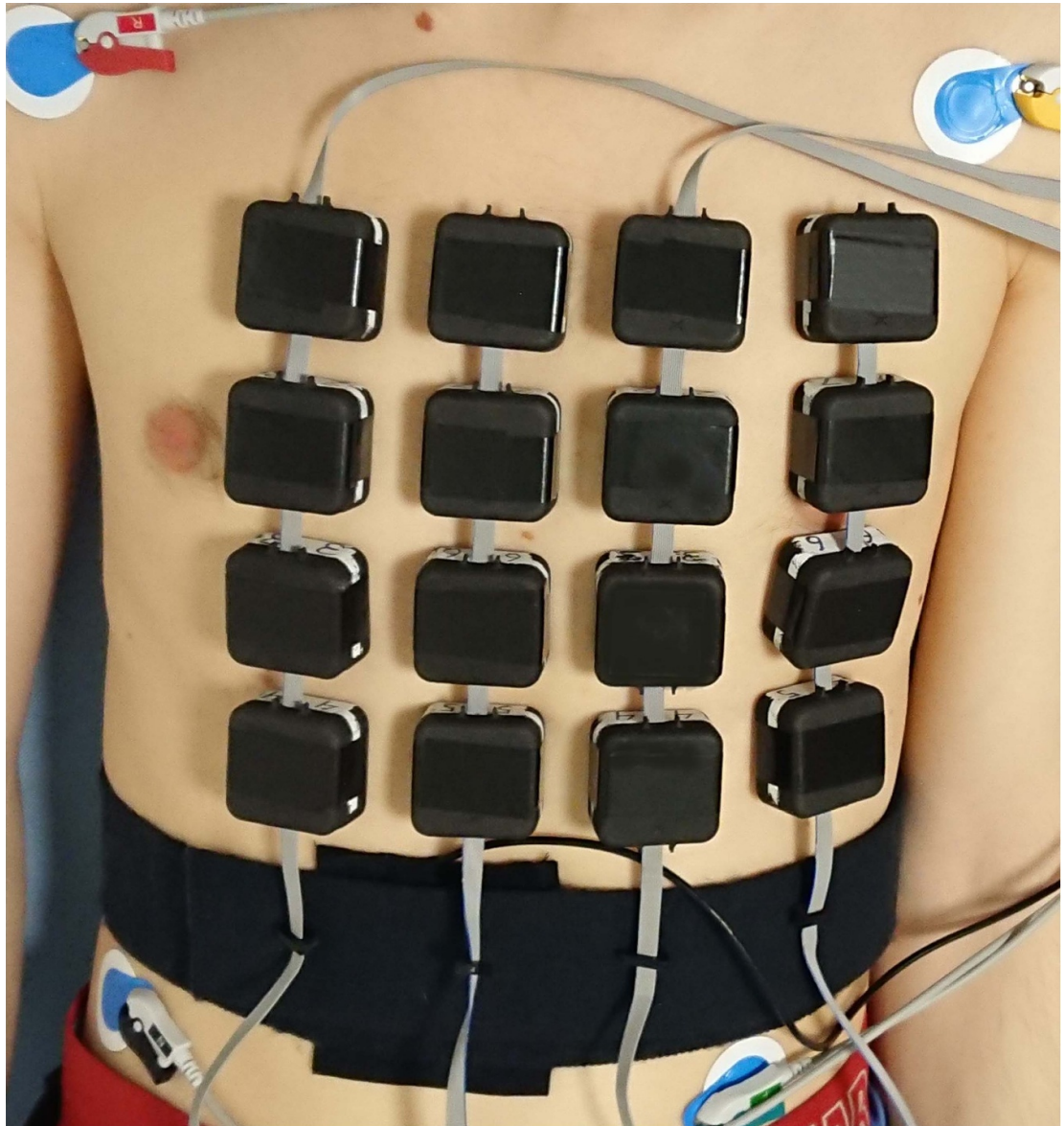
Figure 4. Illustrates the experimental setup human trials. In the corners of the figure are the ECG electrodes, on the chest are 16 sensors, and across the abdomen is a respiration belt.
