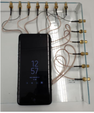
Figure 2. A photo of a commercial LTE mobile handset supporting multi-band 4 \times 4 MIMO.
