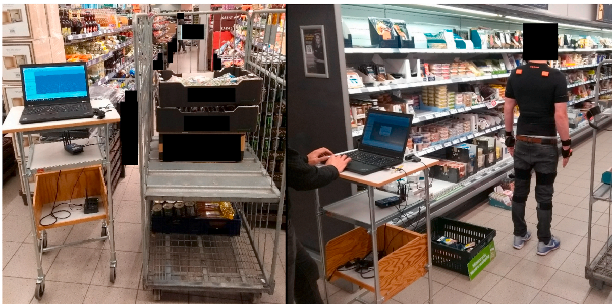
Fig. 1. Left: rolling table with laptop computer, wireless receivers and video camera, and transport cage with shelves. Right: calibration of the motion analysis system before a measurement. The EMG electrodes are hidden under the t-shirt.
