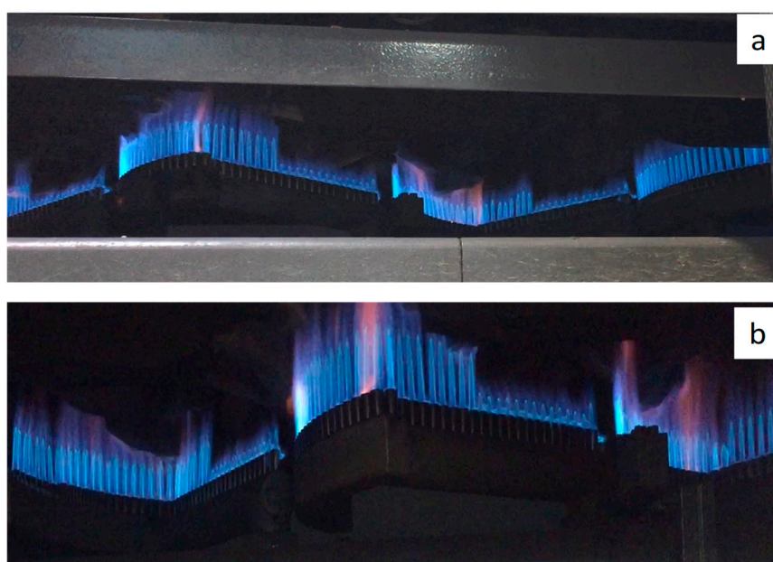
Figure 8. Flame colour before (a) and after (b) combustion air preheating.
