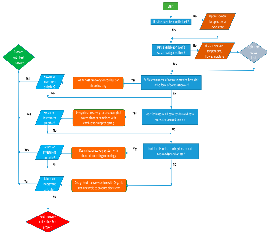
Figure 12. Process map for the selection of suitable heat recovery technology.
