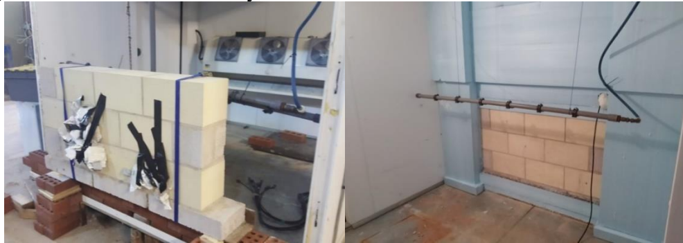
Figure 1. Test wall installed into climate chamber for frost testing. 1a. Exterior, prior to installation. 1b. Interior, after sealing.
