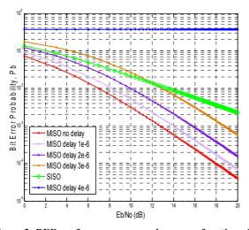
Figure 2: BER performance comparisons as a function of SNR and transmission delay difference in quasi-static flatfading channels.
