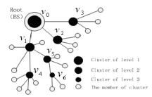
Figure 2. root tree vs. clustering of sensor networks
