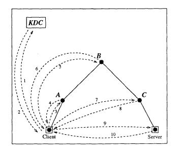
Fig. 4. Authentication with localized keys
