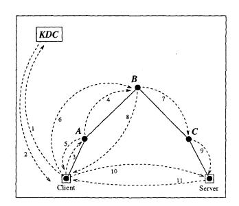
Fig. 5. Authentication with globalized keys
