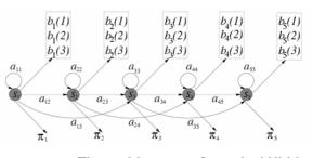
Figure 1 –The architecture of a typical Hidden Markov Model<sup>[12]</sup>
