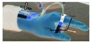
Figure 2 – Mounting of the sensors on hand
