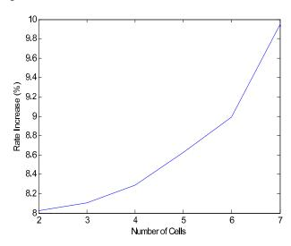
Fig. 5. Total Network Sum Rate with different number of cells, K=256, S=40 and R=4
