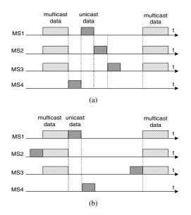
Fig. 1. Scheduling Samples for unicast and multicast traffic
