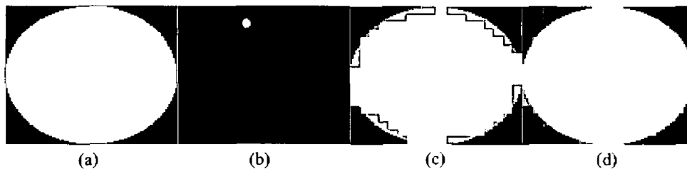
Figure 5: (a) The ball template; (b) The extracted ball shape at 15 \times 22 resolution; (c) match between the template and the extracted ball, where the candidate region is drawn over the template; (d) template is over candidate region.
