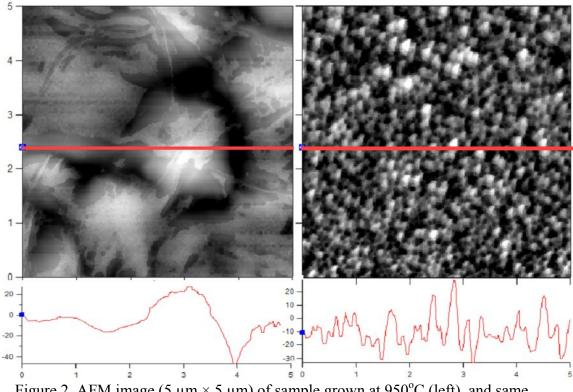
Figure 2. AFM image (5  $\mu$ m × 5  $\mu$ m) of sample grown at 950°C (left), and same sample with Ni as sputtered. Lower portions show height sections along the red lines (in nm).
