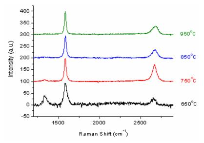
Figure 4. Raman spectra of samples grown at different temperatures.
