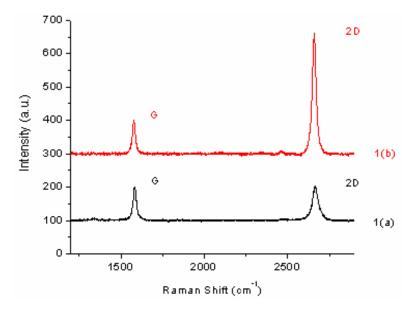
Figure 3. Raman spectra of samples grown at 950°C. On a typical sample spectra like 1(a) occur more frequently than spectra with high 2D/G ratios like 1(b).
