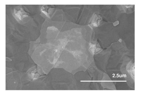
Figure 1. SEM image showing grains of Ni and graphene flakes deposited on it.
