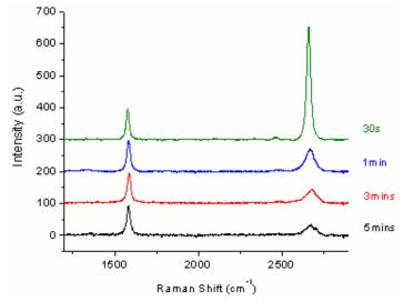
Figure 5. Raman spectra of samples grown at 950°C with different dwell times.
