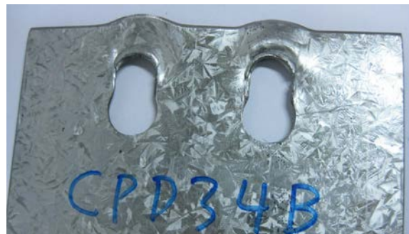
Figure 2. Shear-out of individual bolts
