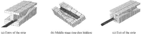
(b) Middle stage (top dies hidden) FIGURE 4. Millipede Forming process of U-channel
