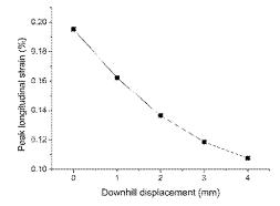
FIGURE 3. Effect of Downhill Displacement on Longitudinal Strain Reduction
