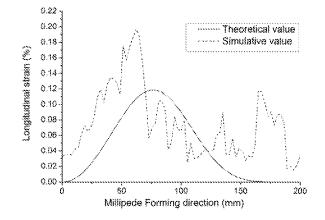
FIGURE 5. Axial longitudinal strains of the flange edge
