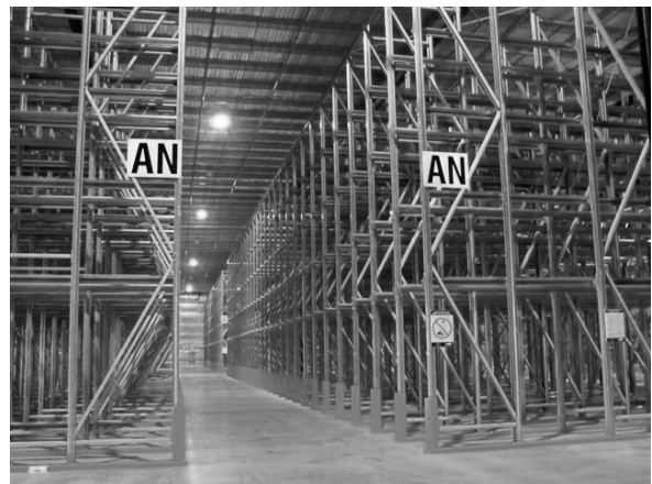
Figure 1: Example of a drive-in rack
