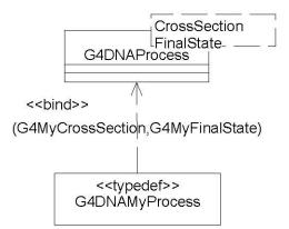
Fig. 2 An example of a template specialization : MyProcess is a specialization of G4DNAProcess.
