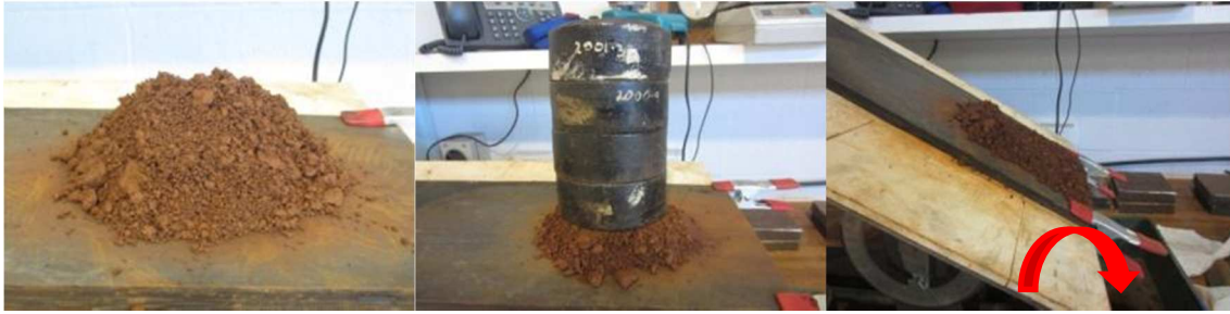
Figure 5 - Example of experiment to calibrate particle-to-wall interactions under static conditions
