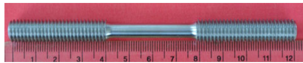
Fig. 1—Dimensions and appearance of tensile specimen used in the current study.
