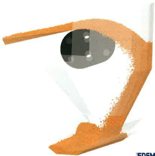
Figure 4: Simulation of a problematic transfer station conveying bauxite at 5000tph.
