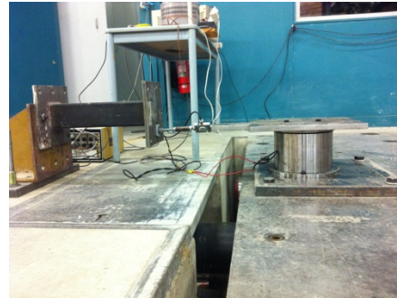
Figure 6 b) Test photo for MRE base isolator prototype 2
