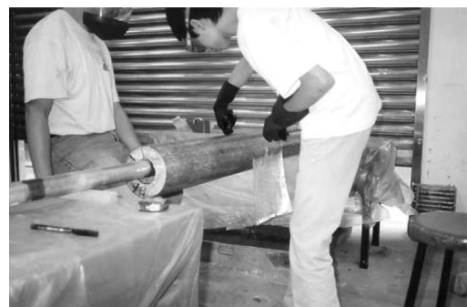
Fig. 5. Fabrication of FRP tube
