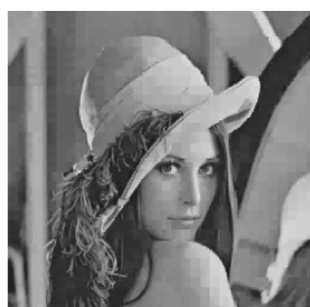
(c) Coded with prediction, Th=0.1 bpp=0.62, PSNR= 30.42
