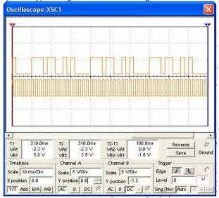
Fig. 7. Decoded output PN sequence and recovered clock waveforms.
