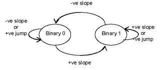
Fig. 3. State transition diagram of the decoder.
