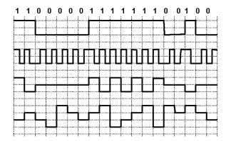
Fig. 2. Example of different encoded waveforms. From top to bottom: NRZ-L, Manchester, AMI, and slope line codes.
