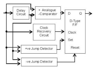
Fig. 6. Slope decoder block diagram.
