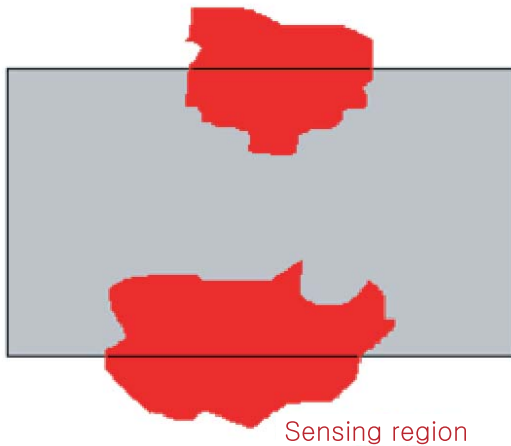
Fig. 13. The sensing region of each sensor node is not uniform. Our Border Coverage algorithm can still work as long as we can find the segment of intersection with the border.
