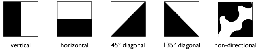
Fig. 3. The 5 edge types used in the edge histogram descriptor.
