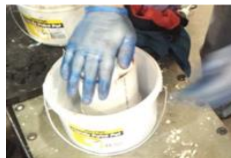
Figure 3b - Moulds pushed into MRC
