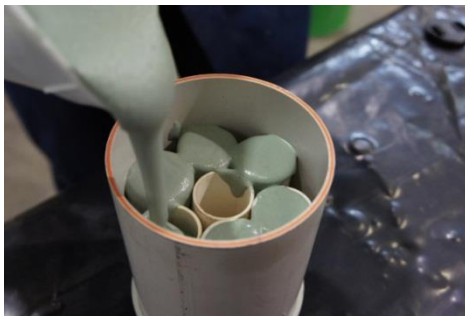
Figure 3a - Mixed resin poured into moulds
