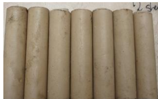
Figure 4 - The process of separating cast samples moulds and removal of individual samples
