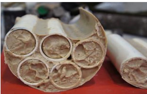
Figure 4 - The process of separating cast samples moulds and removal of individual samples
