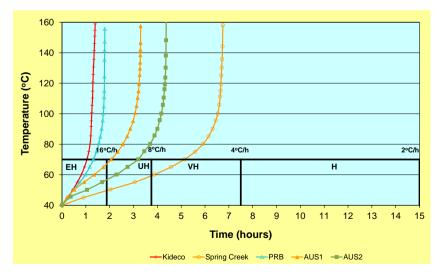
Figure 2 - Adiabatic self-heating curves for samples tested using the normal R<sub>70</sub> test procedure, showing intrinsic spontaneous combustion reactivity ratings based on Queensland conditions (H = High, VH = Very High, UH = Ultra High, EH = Extremely High)
