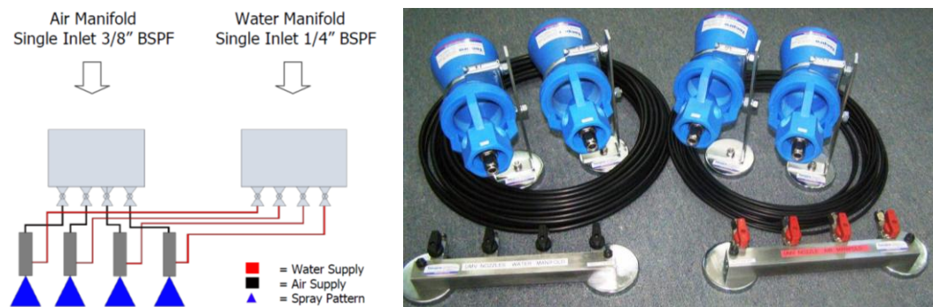
Figure 5 - Air and water coupling pipelines and associated manifold regulating the venturi units and the assembled first prototype unit for field trial
