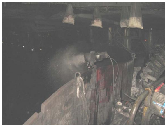
(a) Venturi unit installed on the BSL in the maingate (b) Venturi units installed on MG Chock
