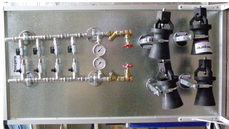
Figure 6 - An assembly of four venturi units made up of fire resistance and antistatic (FRAS) material
