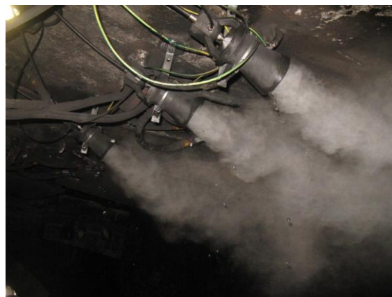
(a) Venturi unit installed on the BSL in the maingate (b) Venturi units installed on MG Chock
