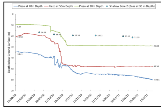
Figure 21 - Piezometer and standpipe for panel 2
