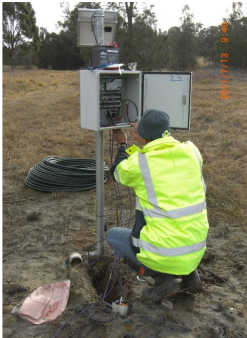
(a) Surface stressmeter system (b) Surface microseismic system Figure 2 - Installation of surface stressmeter and microseismic systems
