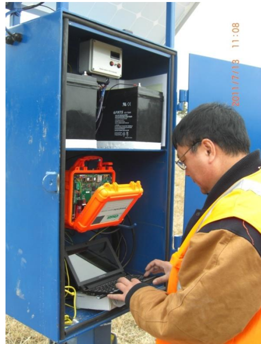
(a) Surface stressmeter system (b) Surface microseismic system Figure 2 - Installation of surface stressmeter and microseismic systems
