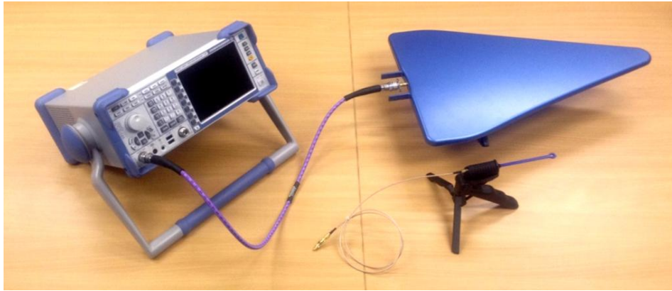
Figure 2 - Test equipment used to measure the electric and magnetic fields radiated from the GPR systems include the spectrum analyser (left), 400 MHz to 6 GHz log periodic antenna (top right), and 12 mm loop antenna (bottom right).
