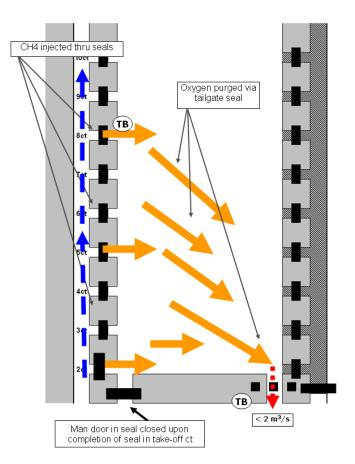
Figure 3 - CH<sub>4</sub> injection via MG seals continues while airflow via TG is reduced
