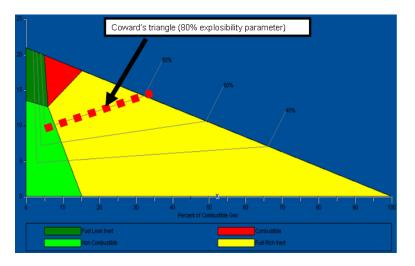
Figure 4 - Coward's triangle showing 80% explosibility parameter
