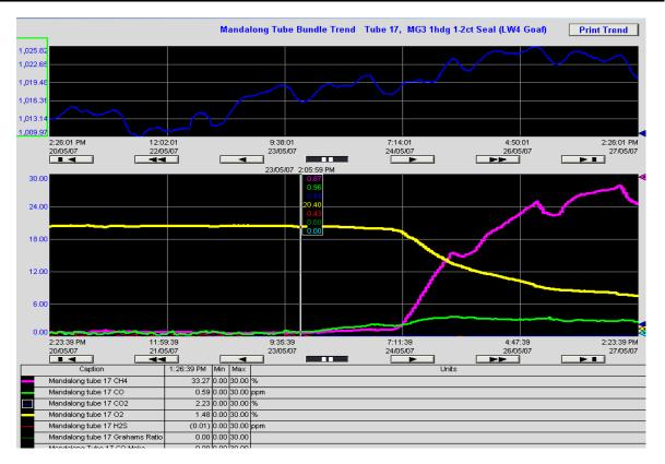
Figure 1 - Self-inertisation trend for LW4 final sealing
