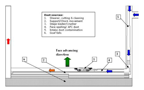
Figure 1 - Sources of dust generation on longwalls
