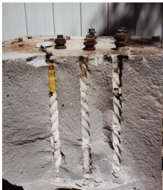
Fig 2 - Rifled drill hole
