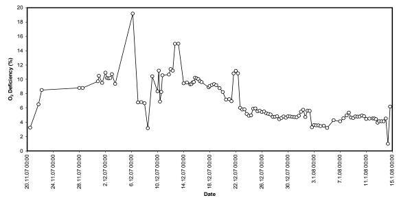
Figure 5 - The variation in O<sub>2</sub> deficiency values for Gelik mine fire incident
