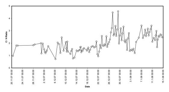
Figure 8 - The variation in C/H ratio for Gelik mine fire
