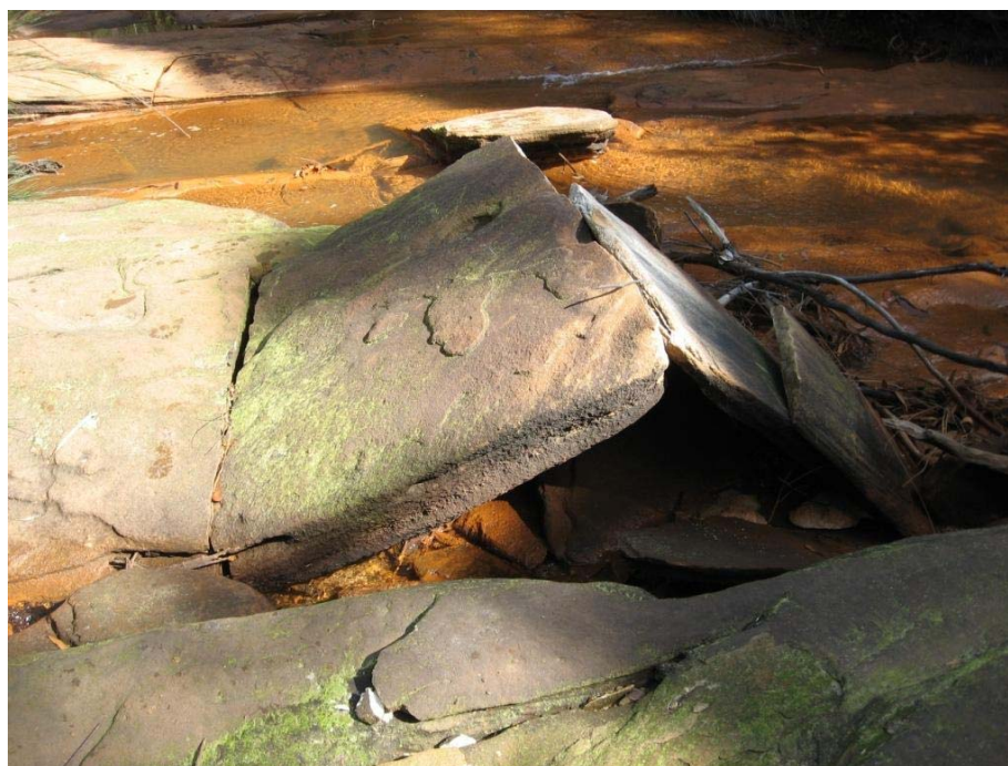
Figure 2 - Buckling of near-surface, Waratah Rivulet, late 2004
