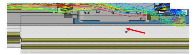
(a) Plan view of dust particle capture and flow patterns - scrubber discharge at 10° towards the face
