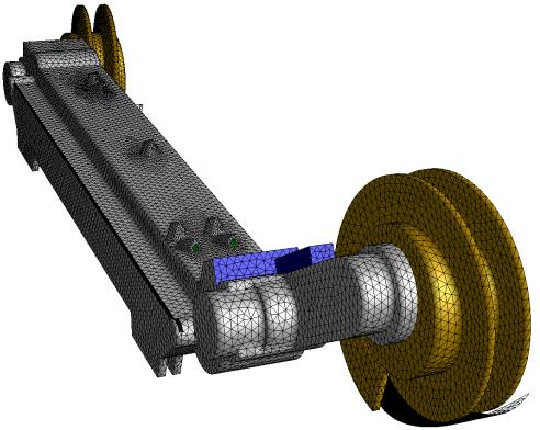
Figure1 - Computational mesh of the CFD model - the longwall shearer
