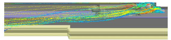
(b) Shearer clearer induced airflow – 0.25 m<sup>3</sup>/s
