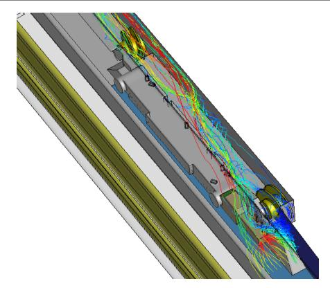
(b) 3D view of dust particle capture and flow patterns - scrubber discharge at 10° towards the face
