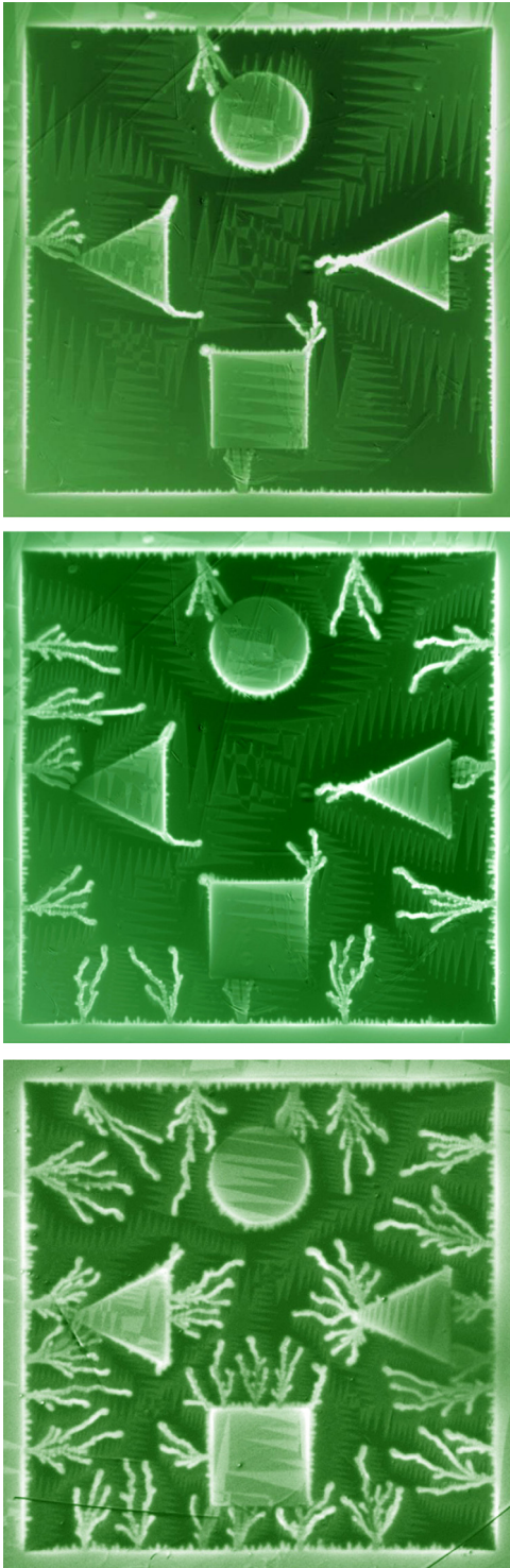
FIG. 3. Images of the flux distribution in a sample with differently shaped holes. After initial zero-field cooling, the images were taken at applied fields of 2.25 mT (upper), 3.15 mT (middle), and 4.20 mT (lower).
