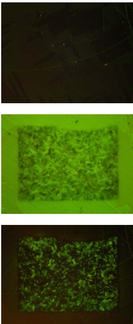
FIG. 5. (Color online) Magneto-optical images on the polycrystalline sample. Top: image taken at external field of 8 Oe showing Meissner state after ZFC. Middle: imaging taken at 160 Oe showing flux penetration easily along intergranular path. Bottom: remanent state after field increased to 800 Oe and decreased to zero.
